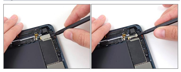
• Use the tip of a spudger to lift up the lower side of the metal bracket.
