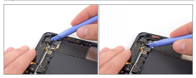
• Straighten the rear-facing camera ribbon cable to expose the camera housing.
