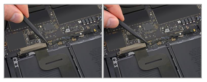
Pry up and disconnect the locking flap on the connector at the opposite end of the battery board data cable.
