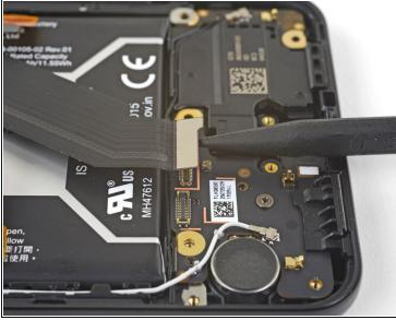
Use the point of a spudger to pry up and disconnect the interconnect cable from its daughterboard socket.
