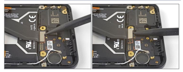
• Use the point of a spudger to pry up and disconnect the interconnect cable from its daughterboard socket.
