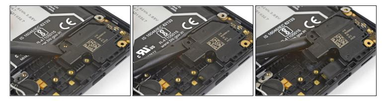
(i) The loudspeaker itself is adhered to the phone frame near the right edge of the phone.
