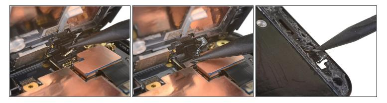
This step shows how to reconnect the proximity sensor during re-assembly.
