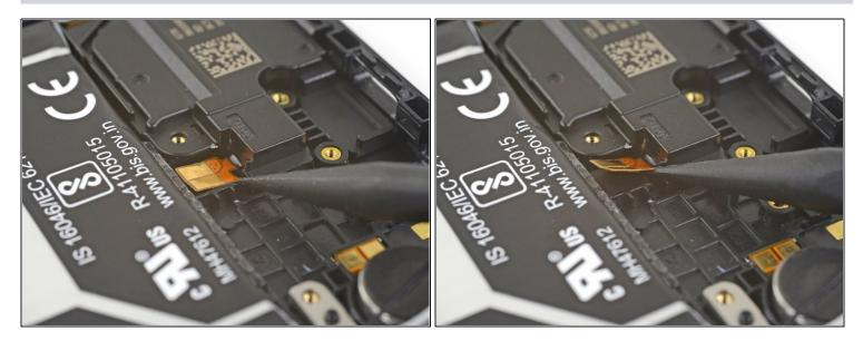
• Slide the point of a spudger underneath the loudspeaker's flex contact pad and pry it loose from the phone frame.
