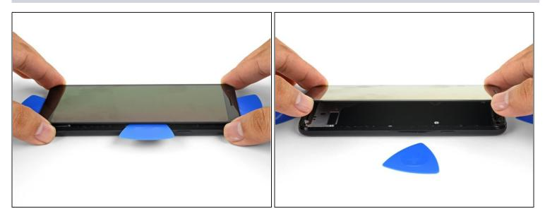
• With all of the edges cut, carefully hinge open the **right edge of the screen**.
