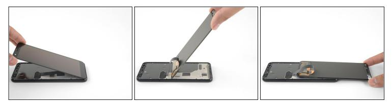
• With all of the adhesives cut, flip the attached screen glass side down and rest it on top of the phone. The screen flex cable should be loosely arched.
