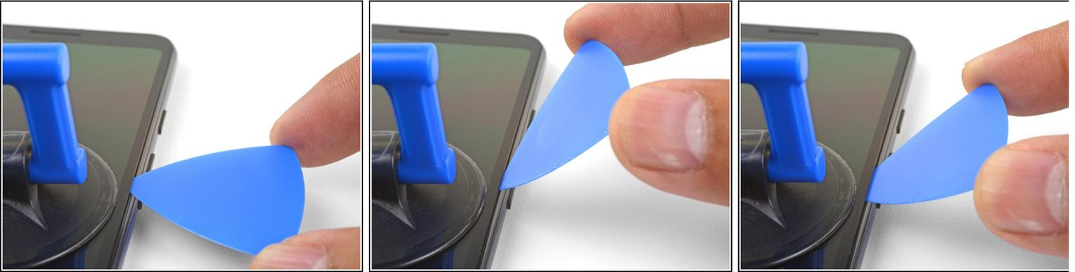
**i** This step shows how to insert the pick without damaging the OLED panel. Do this before you slice either long edges of the phone.
