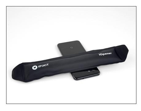
• Heat an iOpener and apply it to the fingerprint sensor for a minute. This will soften the adhesive holding it in place.
