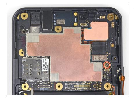
Remove the single 2.7 mm T3 screw securing the motherboard near the right edge.
