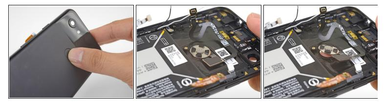
• Use your finger to press against the fingerprint sensor from the back of the phone until it loosens from its cutout.
