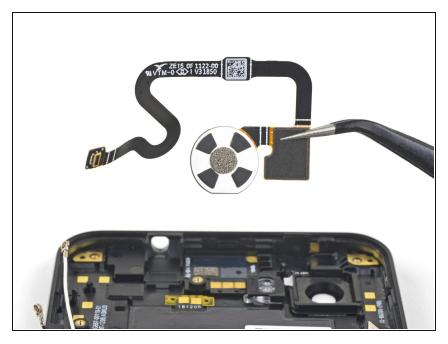
• Remove the fingerprint sensor.
