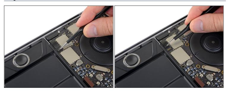
• Peel back any tape covering the connector for the left-side tweeter.
