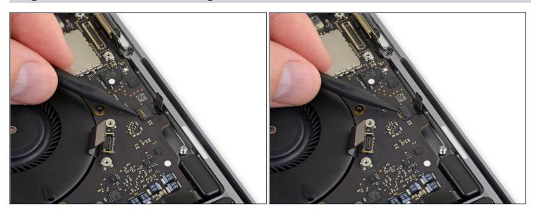
• Open the locking flap on the microphone cable's <u>ZIF connector</u> by prying it straight up from the logic board.
