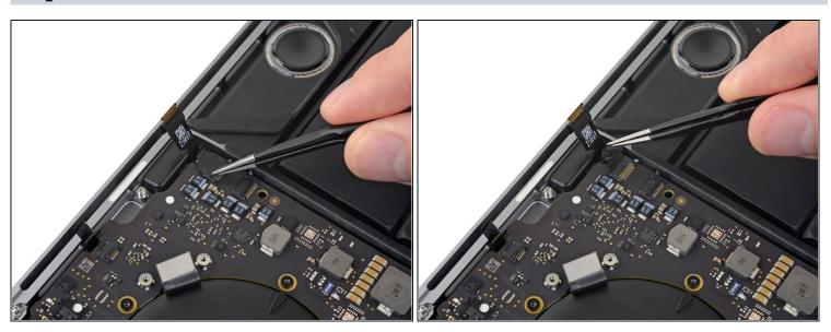
• Peel back any tape covering the connector for the right-side main speaker.
