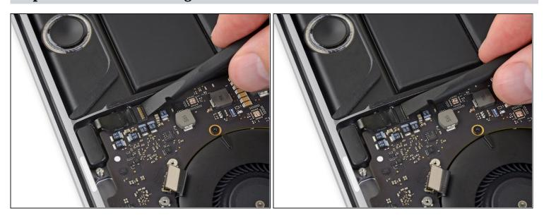
• Flip open the locking flap for the right-side tweeter ZIF connector by prying it straight up from the logic board.
