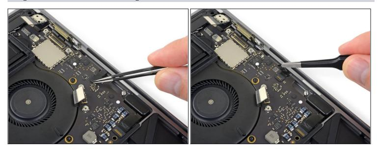
• Peel back any tape covering the microphone connector socket.
