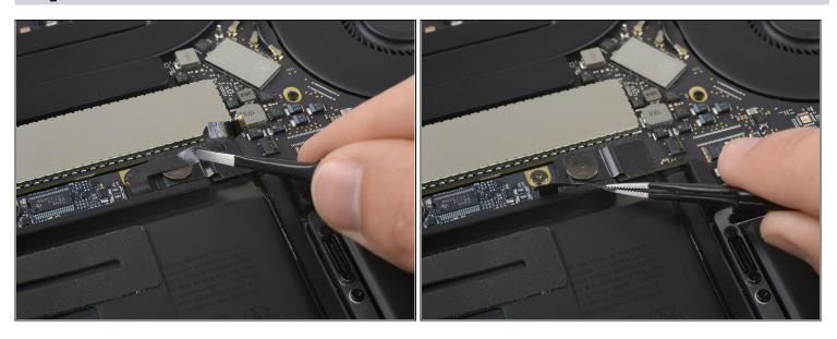
• Fold the battery board data cable to the side and out of the way.
