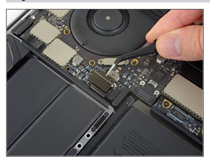
• Remove the keyboard connector bracket.
