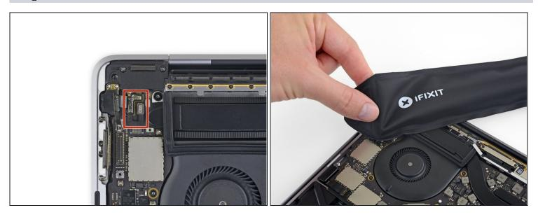
• Apply mild heat using an iOpener, heat gun, or hair dryer to soften the adhesive under the power button/Touch ID flex cable.
