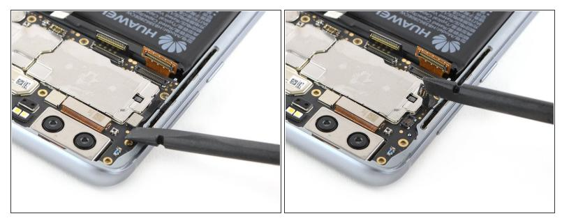
• Use a spudger to pry up and disconnect the power and volume button flex cable.
