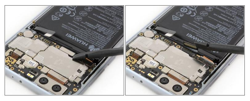
• Use a spudger to pry up and disconnect the interconnect flex cable.
