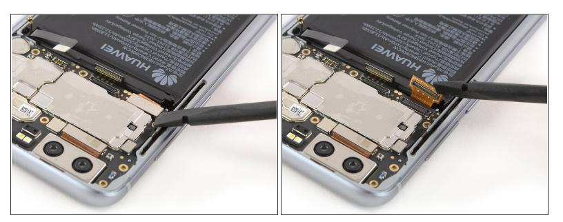
Use a spudger to pry up and disconnect the display flex cable.
