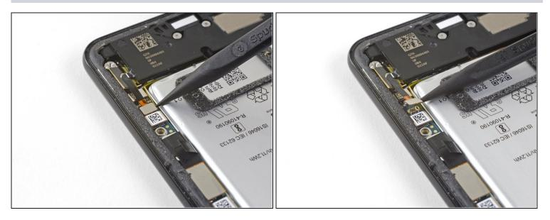
• Use the point of a spudger to pry up and disconnect the loudspeaker connector from its motherboard socket near the right edge of the phone.
