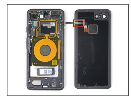
When inserting an opening pick above the power button, be careful not to insert the pick too deeply, or you will damage the fingerprint sensor cable.
