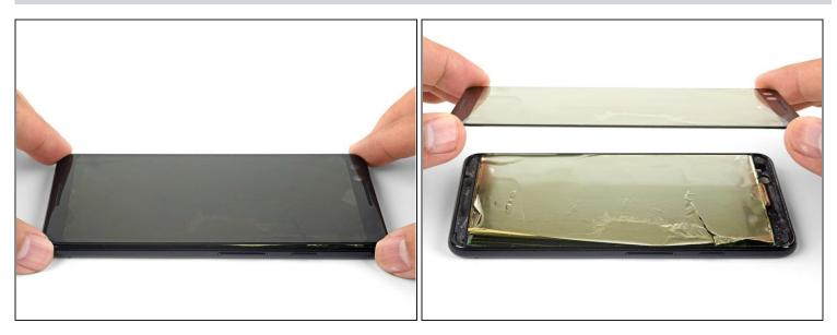
• Lift up and remove the front glass from the phone.
