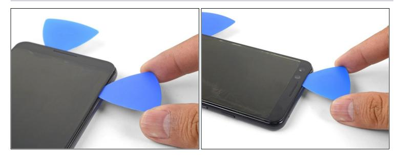
• Continue heating edges with an iOpener and slicing the adhesive with an opening pick, until you've sliced through all of the adhesive.
