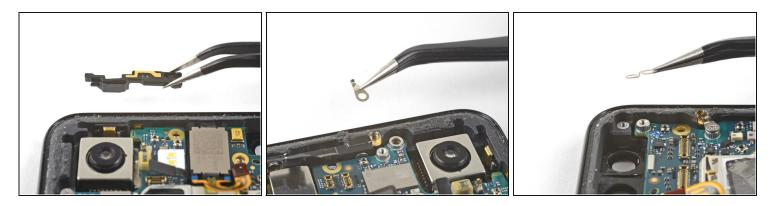
• Carefully remove the antenna bracket from the top left edge of the phone.
