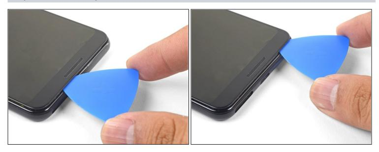
• Slide the pick along the bezel to slice through the adhesive.
