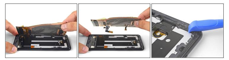
• Thread the screen cable and digitizer cable out of their cutouts, then remove the display.
