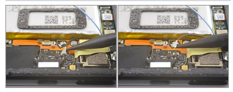
• Use the point of a spudger to pry up and disconnect the black antenna cable from its socket near the USB-C port.
