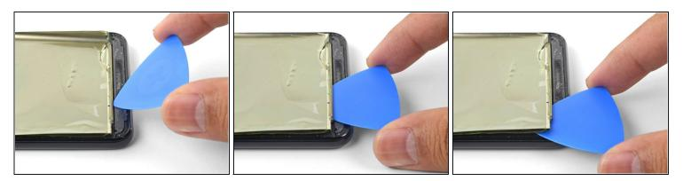
(i) The remaining part of the screen is affixed to the phone frame by a large patch of adhesive.
