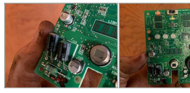
Caps replaced. Bend them slightly forward so they fit inside the opener casing. And reinstall in reverse. Reinstalled after replacing caps and now my garage door functions like it should! I read some reviews off liftmaster's site for the 888LM and many complain of its short life and replacement.
