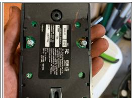
This is the door opener, 888LM. I had a constant red/yellow light blinking and a beep coming from the unit. Replacing the garage door opener main board, did not change anything. (screw is marked)
