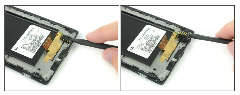
Insert a <u>nylon spudger</u> into the auxiliary port and gently pry upward to free the port.
