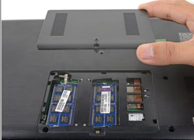
Lift up the edge of the RAM cover and remove it.
