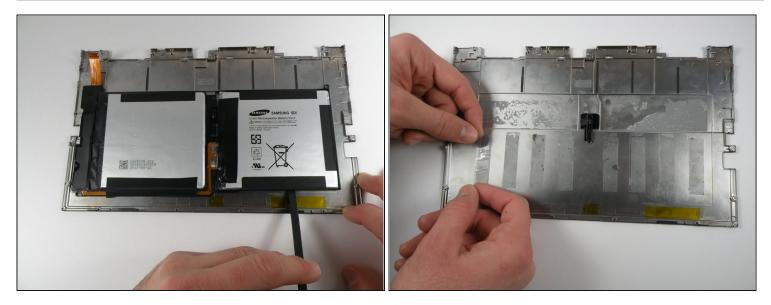
(i) The battery is glued to the back cover but can be easily removed with a spudger
