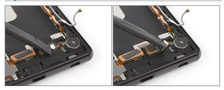
• Use a spudger to pry up and disconnect the vibration motor connector.
