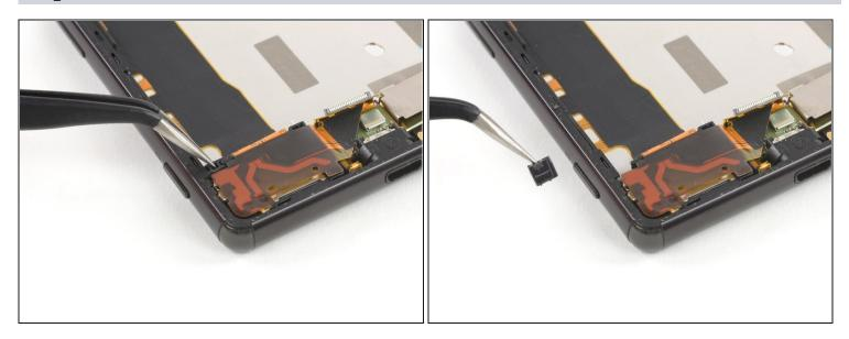
• Also remove the plastic safeguard between the midframe and the loudspeaker cover.
