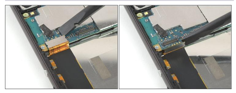
• Use a spudger to pry up and disconnect the side button flex cable on the left side of the motherboard.
