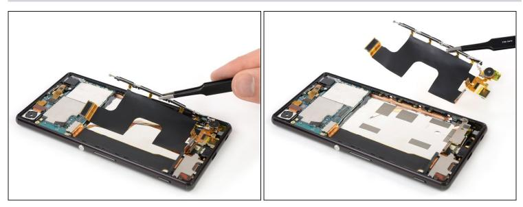
Use a pair of tweezers to remove the main flex cable assembly including the vibration motor and the microphone.
