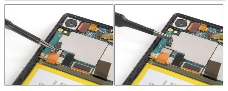
• Use a pair of tweezers to peel the black adhesive strip off the battery connector and fold it out of the way.
