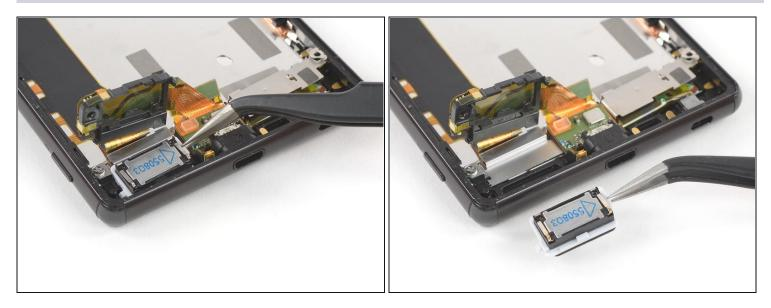
• Use a pair of tweezers to lift the loudspeaker out of its recess and remove it.
