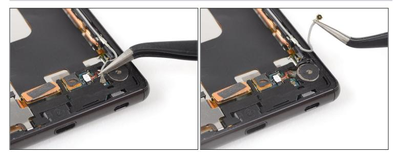
• Use a pair of tweezers to pry up and disconnect the antenna cable.
