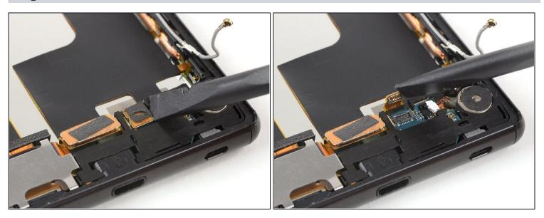
• Use the flat end of a spudger to pry up and disconnect the small main flex connector next to the vibration motor connector.
