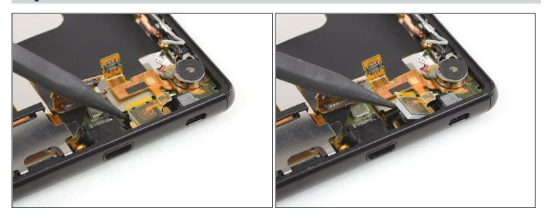
Use the pointed end of a spudger to lever the microphone out of its recess.
