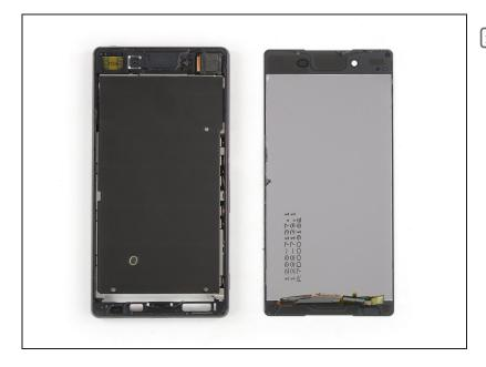
Remove any remaining adhesive from the midframe, and clean the glued areas with isopropyl alcohol and a lint-free cloth before installing a new screen.
