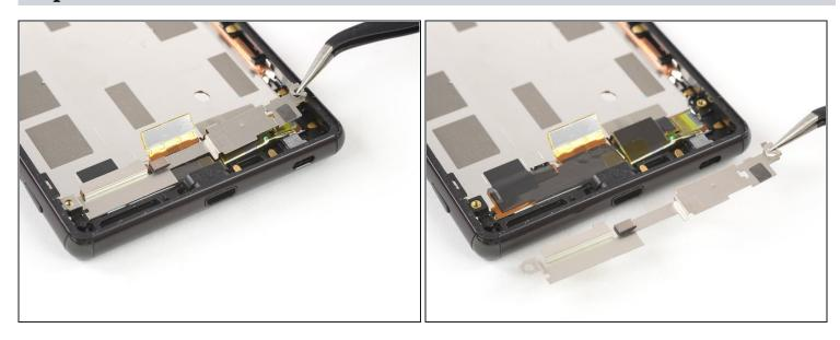
• Use a pair of <u>tweezers</u> to unhook the metal shield on top of the display cable assembly and remove.
