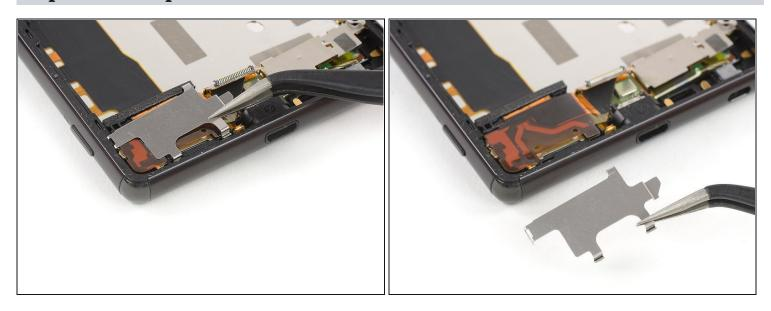
• Unhook and remove the metal shield above the loudspeaker cover located at the bottom left.
