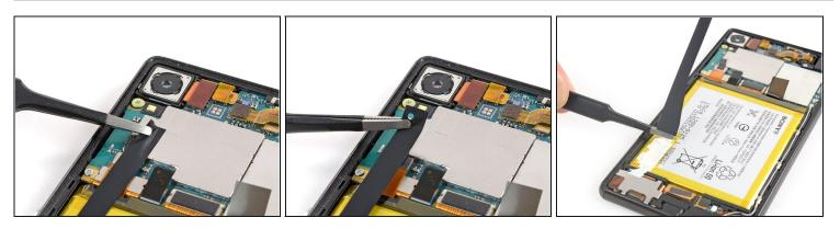
• Use a pair of <u>tweezers</u> to carefully peel the adhesive strip off the mother board and the battery and remove it.
