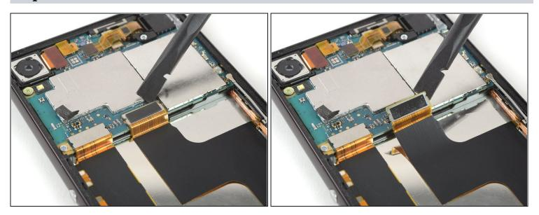
• Use a spudger to pry up and disconnect the main flex cable from the motherboard.
