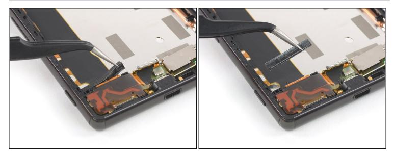
Peel off and remove the foam pad next to the loudspeaker cover.
