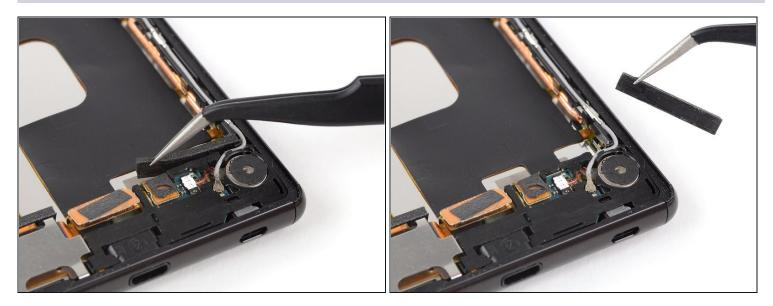
• Use a pair of <u>tweezers</u> to peel off and remove the foam pad on top of the daughterboard.
