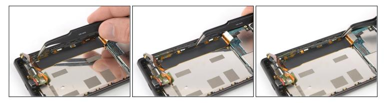
• Use a pair of tweezers to loosen the plastic clips along the side button flex cable on the left side of the midframe.
