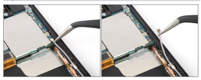
• Use a pair of <u>tweezers</u> to pry up and disconnect the upper connector of the antenna cable.
