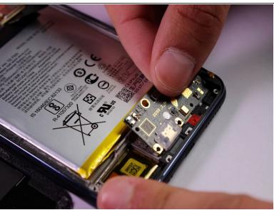
Insert a plastic prying tool on the left side of the charging port. Gently lift up the charging port and then remove using your hand.
