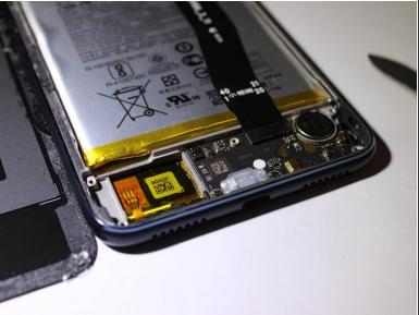
Use the nylon spudger to pry off the lower cover. Use the opening tool to help lift it off.
