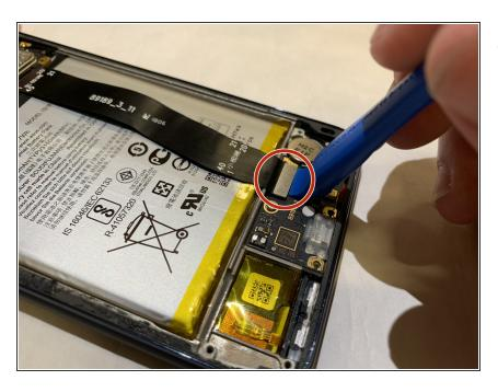
Pop out the connector that goes over the front of the battery and use the iFixit opening tool to remove it from the circuit board.
