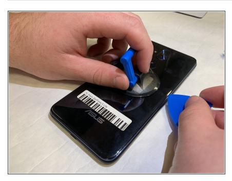
Remove the back cover of the phone with the suction cup and opening picks.
