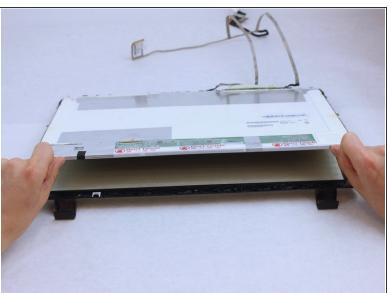
• Lift the backlight panel out and replace it.
