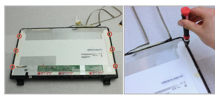
Remove the six 3 mm Phillips #00 screws from the backlight frame.
