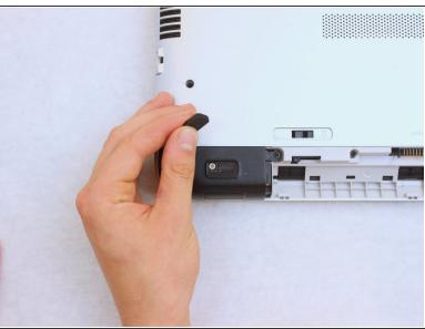
Remove the rubber feet on each corner cover with a plastic spudger or plastic opening tool.
