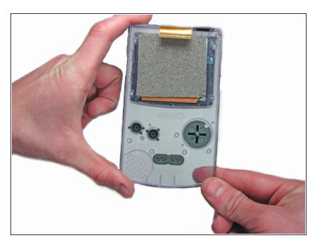
Remove the original buttons from the housing.
