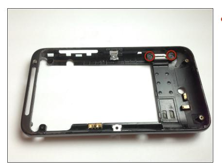
Remove the two Phillips screws on the bottom right of the rear frame.
