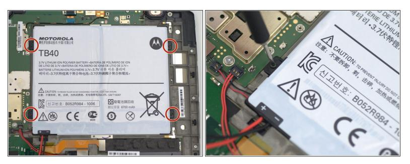
Using a Torx T5 screwdriver, remove the four 1.5mm screws holding down the battery around its perimeter.
