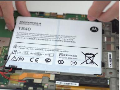
Using the opening picks, carefully lift the battery and remove it from the device.
