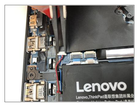
Using a pair of tweezers, push the sides of the white speaker wire toward the battery (where it says Lenovo) to unplug it.
