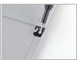
To open the hinge, insert your T5 Torx screwdriver into one of the screw holes and gently pry
