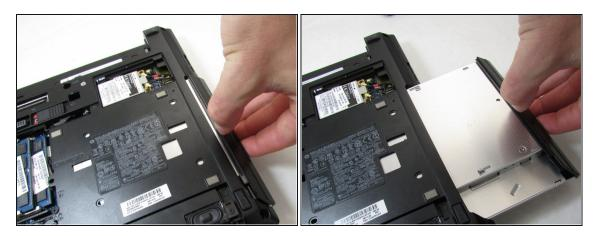
With your fingernail, pry the edge of the optical drive away from the chassis of the laptop and pull it straight out.
