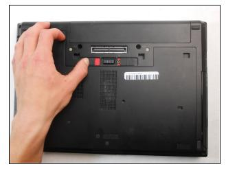
On the back of the computer, slide the left switch towards the outside of the laptop until you hear a click.
