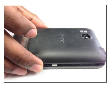
• Lift and remove the rear panel.
