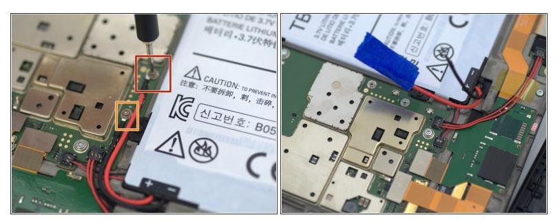
Disconnect the battery first for safety by unscrewing the two 1.5mm screws with a T5 Torx screwdriver.
