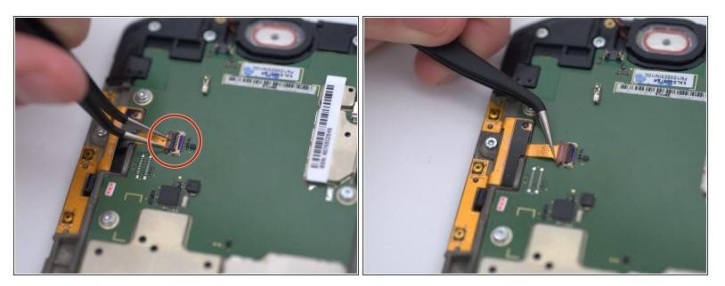
Using a pair of tweezers, carefully pry up the black plastic connector holding the cable.
