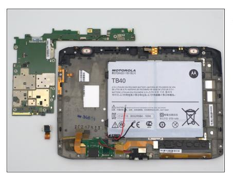
• Remove the motherboard from the device.
