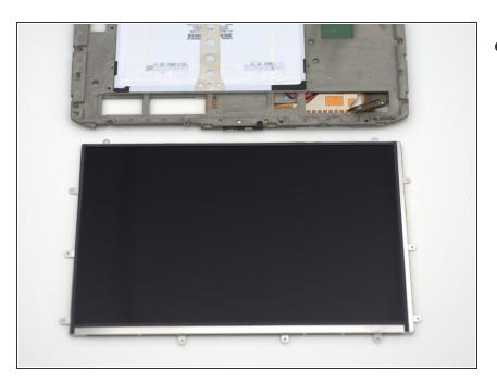
Remove the LCD from the device.
