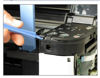
Using the plastic opening tool, gently pry around the button cover to remove it from its fixture.
