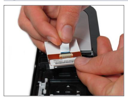
Gently pull the ribbon cable to remove the LCD completely.
