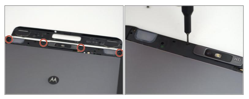
Using a T5 screwdriver, unscrew the four 1.5mm screws holding the main back cover. These screws are arranged in a line across the top of the back of the device.
