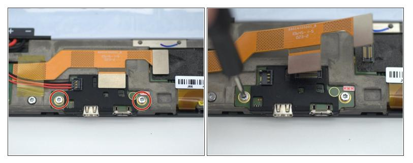
Using a Torx T5 driver bit, unscrew the two 1.5mm screws holding down the charging port assembly.
