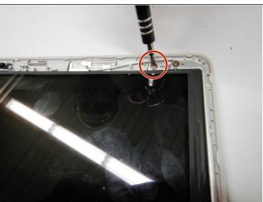
Use the Phillips #1 screwdriver to remove the four 3.0 mm screws securing the screen to the top cover.
