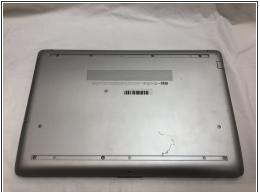
Using the plastic opening tools, peel back the plastic feet from the underside of the laptop.
