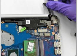
Carefully use the metal tweezers to remove the display connection to the motherboard.
