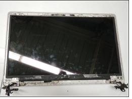
Starting from the area near the hinges, gently remove the adhesive display bezel from around the screen using the iFixit opening tool.
