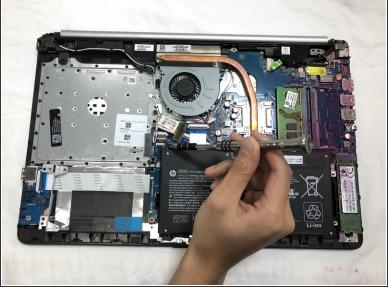
• Using the Phillips #1 screwdriver, remove the three 8.0 mm screws holding the battery in place.
