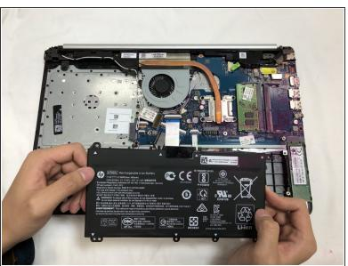
Remove the battery by tilting the top of the battery towards you and pulling the battery away from the mounting tabs.
