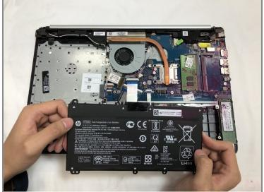
Remove the battery by tilting the top of the battery towards you and pulling the battery away from the mounting tabs.
