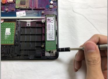
Using the Phillips #1 screwdriver, remove the single 3.0 mm screw holding the SSD module in place.
