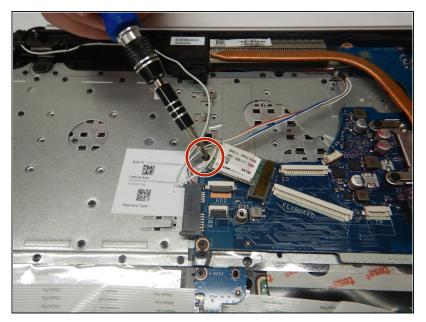
Using the Phillips #1 Screwdriver, remove the single 3.0 mm screw holding the wifi card and gently pull the wifi card away.
