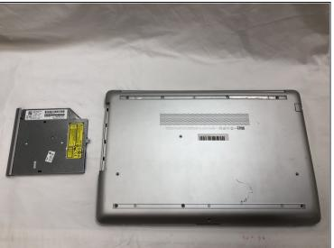
Slide the optical drive out of the computer.
