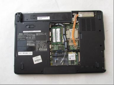
• Use a Phillips #0 screwdriver to remove the eight 3mm screws from the rear casing of the laptop.
