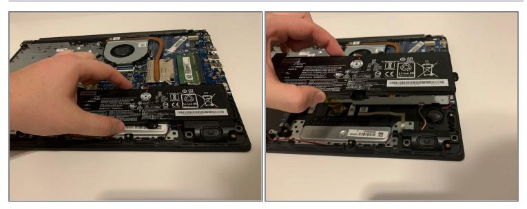
• Grabbing the sides of the battery with one hand, remove the battery from the laptop.
