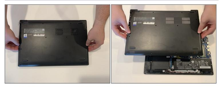
i Make sure that the back panel is completely free from the laptop.
