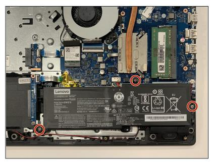
• Using a Phillips #0 screwdriver, remove three 6.0mm screws.
