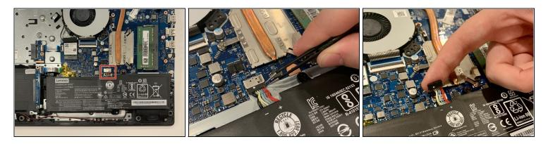
Using a pair of tweezers, remove the black plug which includes 8 wires.
