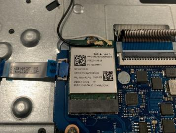
Using a plastic opening tool, lift the black tab to remove the blue tab from the Motherboard.
