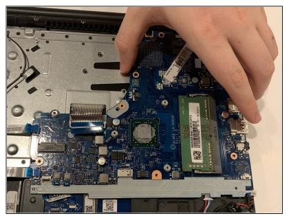
• Lift up and remove the motherboard from the device.
