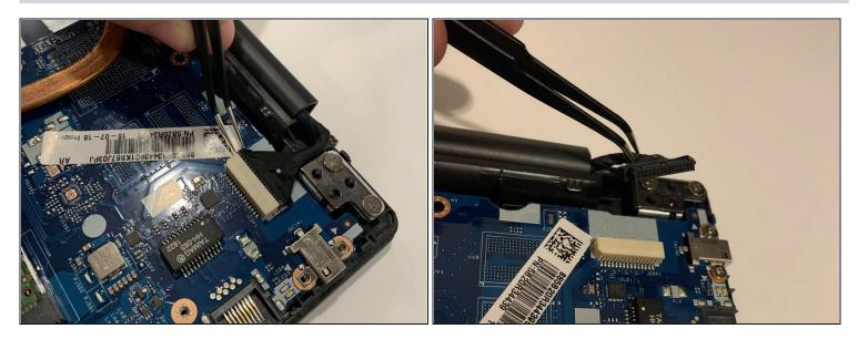
• Using a pair of tweezers, remove the plug from the motherboard.
