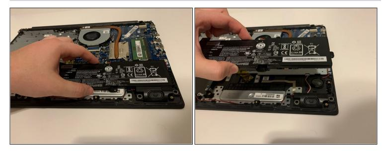
• Grabbing the sides of the battery with one hand, remove the battery from the laptop.
