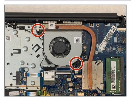
Using the Phillips #0 screwdriver, remove two 4.0mm screws.
