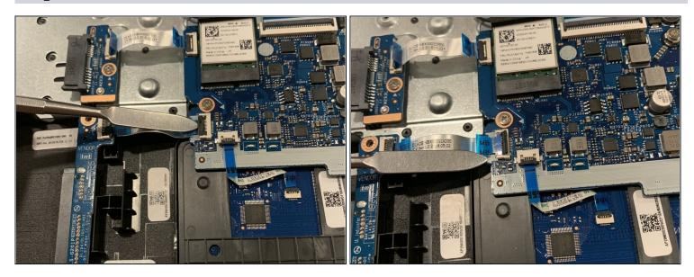
Using a plastic opening tool, lift the black tab to remove the blue tab from the Motherboard.
