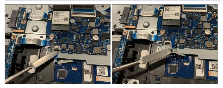
• Using a spudger, lift the black tab to remove the blue tab from the Motherboard.
