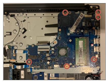
Using a Phillips #0 screwdriver, remove six 6.0mm screws.
