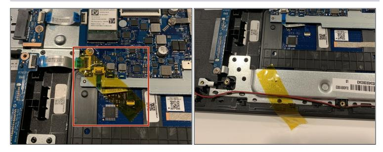
• Remove the yellow tape from the motherboard to ensure freedom of movement upon removal.
