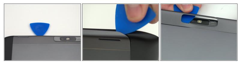
Pry off the silver top back cover (the panel around the camera) with iFixit opening picks or a similar implement.
