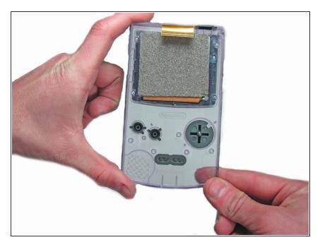
Remove the original buttons from the housing.
