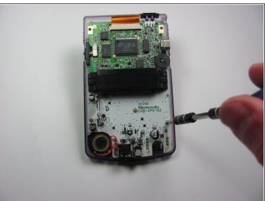
Using the Phillips #1 screwdriver, remove the 3 screws shown in the picture.
