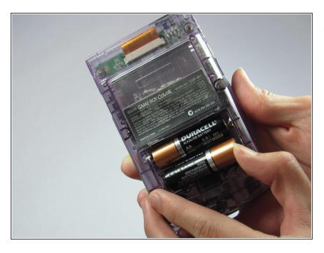
Remove the batteries from the battery compartment.
