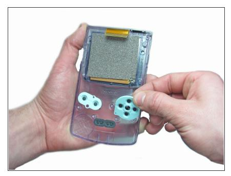
Remove the rubber backing on each button grouping.
