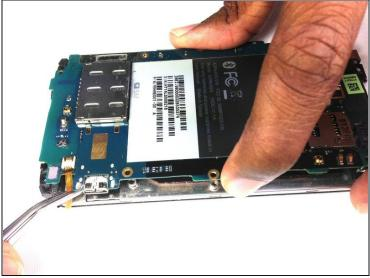
• Using the tip of an plastic opening tool flip up the tab holding the capacitive button ribbon cable.
