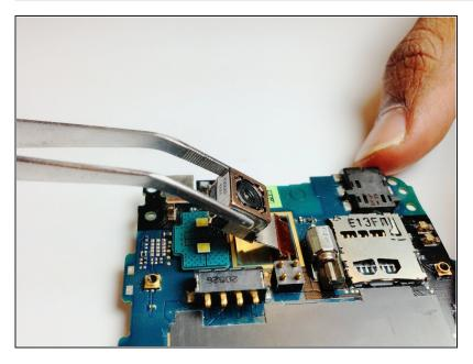
Flip over motherboard and using tweezers gently grab the camera, then pull back and up.
