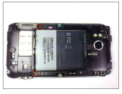
Remove the two Phillips screws securing rear inner frame to device.
