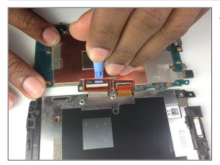
Using the plastic opening tool pop up the two tabs connecting the LCD and motherboard.
