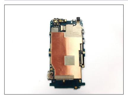
The motherboard should now be completely disconnected
