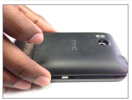
• Lift and remove the rear panel.
