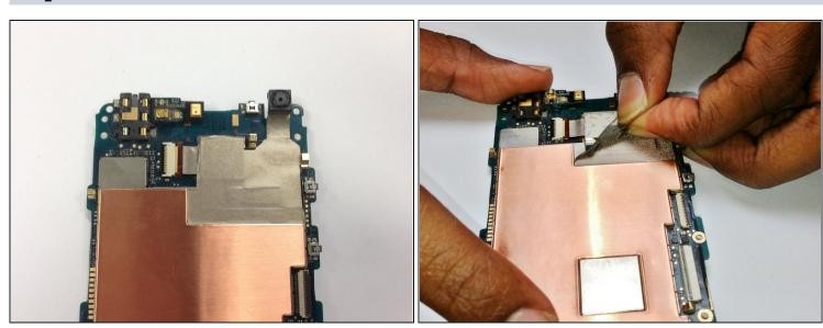
• Use a finger nail to get in between the tape and the phone, then pull the tape off gently.
