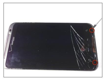
Remove the two Phillips screws where the plastic cover was.
