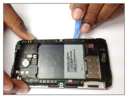
Insert the plastic opening tool between the rear inner frame and the motherboard and slowly work your way around the device.
