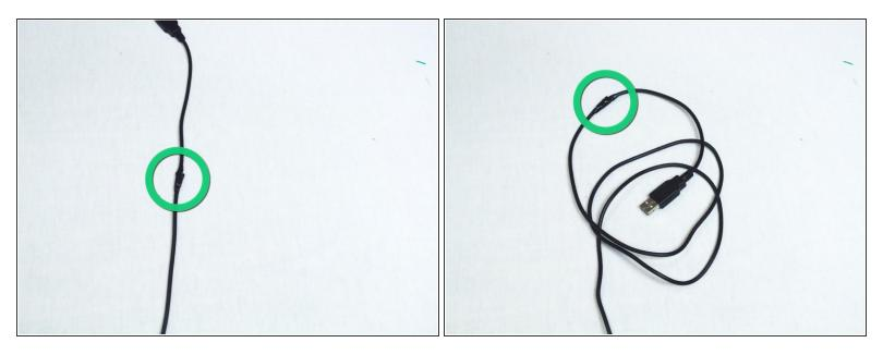
• Wrap all the wires and both cables together in electrical tape to connect everything back into one cable and so it lasts longer.
