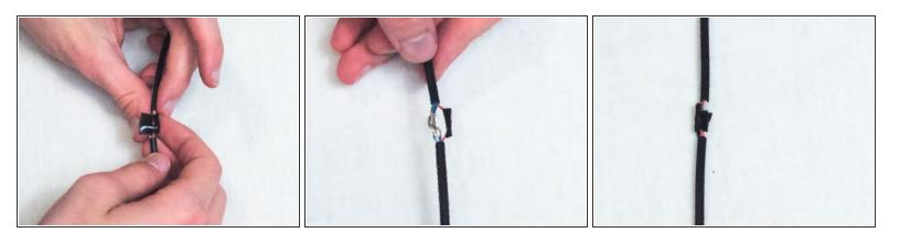
• Wrap each wire in electrical tape and make sure that there is no exposed copper showing.
