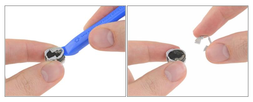
Use a plastic opening tool to pry up and remove the crescent-shaped cap on the top side of the battery housing.
