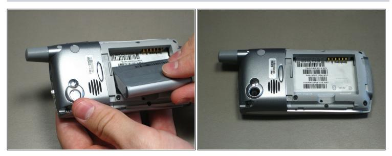
• Lift the edge of the battery, separating contact points, and pull out as pictured.
