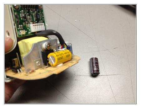
Resolder new capacitor in place, noting the correct polarity.
