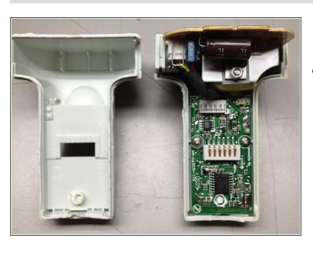
Using a spudger or similar stiff plastic tool, begin prying around the unit in the line that you previously scored, avoid having the tool go in to the device and damaging components. Eventually it will split apart.
