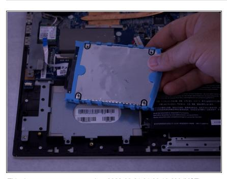
Lift the hard drive from the device.
