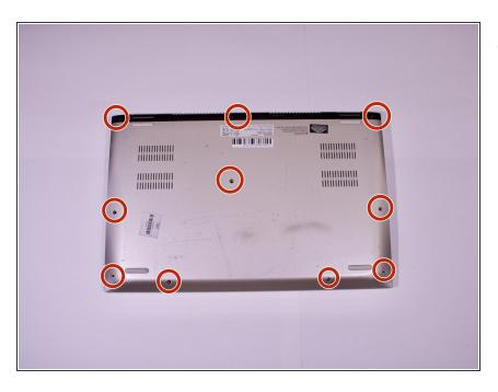
Use a Phillips #00 screwdriver to remove the 10 screws that secure the back cover to the device.
