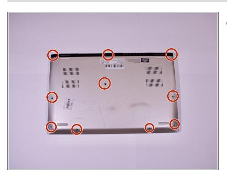
Use a Phillips #00 screwdriver to remove the 10 screws that secure the back cover to the device.
