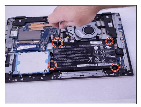
Using a Phillip's #00 screwdriver, remove the four 7.0 mm screws that secure the battery to the motherboard.
