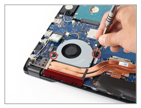
Using a Phillips #1 screwdriver, remove the two indicated 4 mm screws from the other gray fan.
