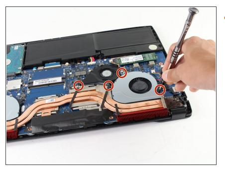
Using a Phillips #1 screwdriver, remove the four indicated 4 mm screws that hold the black fan and the silver one adjacent to it.
