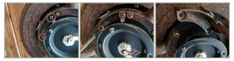
Remove the two screws securing the broken blade arm. Then separate the broken component from the fan.
