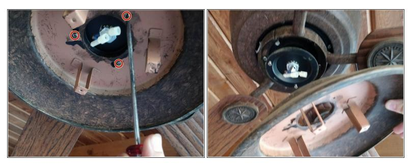
Remove the three screws from the fitter plate. This will allow the plate to easily be separated from the fan.
