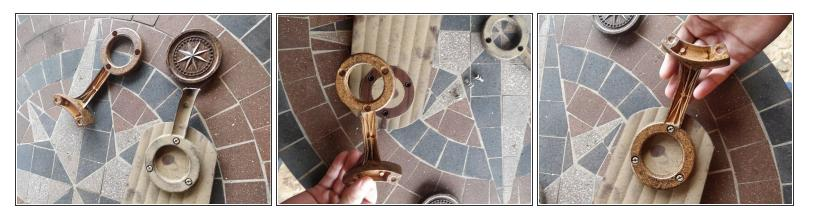
Replace the broken blade arm on the fan blade. There are two components that are placed on either side of the blade and secured together with screws.
