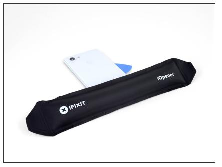
• Apply a heated iOpener to the bottom of the back cover for a minute.
