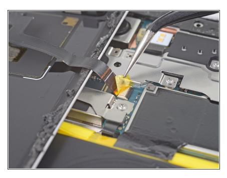
User tweezers to carefully peel up the yellow tape over the fingerprint sensor connector.
