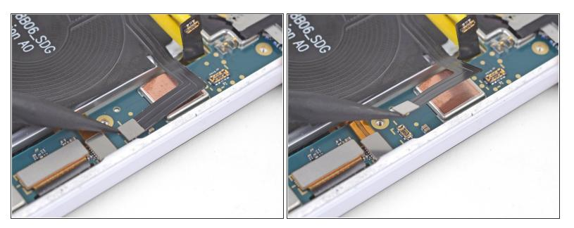
Use the point of a spudger to pry up and disconnect the charging coil connector from motherboard near the right edge of the phone.
