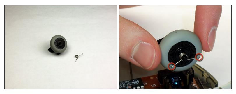
Place the replacement spring on the correct side of the wheel (shown in the images) with the prongs pointing down.
