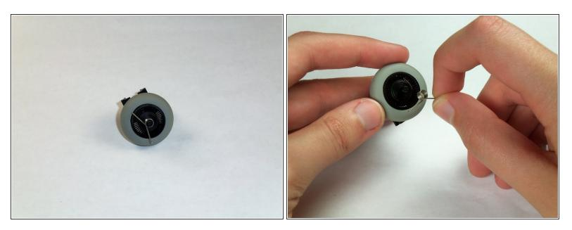
• Locate the spring on the scroll wheel, and carefully remove the spring.
