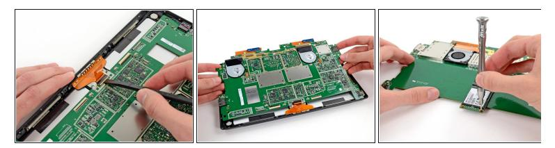
• We've cracked the surface (figuratively speaking, of course—we would never damage a device...), but we continue digging deeper with our <u>spudger</u> and screwdriver until we can remove the motherboard assembly and the SSD.
