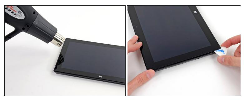
• We are starting to miss the <u>old Surface</u>, as we find a metric <u>duckload</u> of adhesive holding the screen in place.
