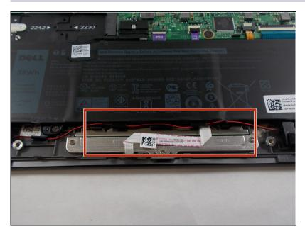
Uncoil the wire connecting the left and right speaker from around the bottom of the battery.
